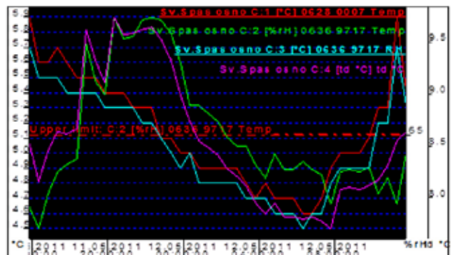
Fig.4–The measurement from the 4 measuring points in the interior ambient of the church on the solemn liturgy (11.05 till 12.05.2011)
